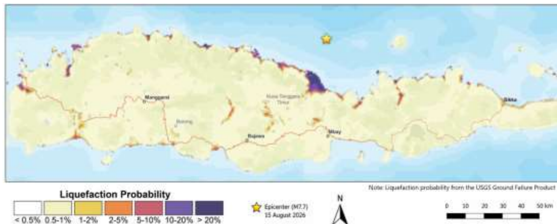
Figure 3. Liquefaction hazard following the 2026 Flores earthquake
